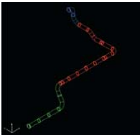
In Version 5.3 you can automatically split the pipes for isometric generation
