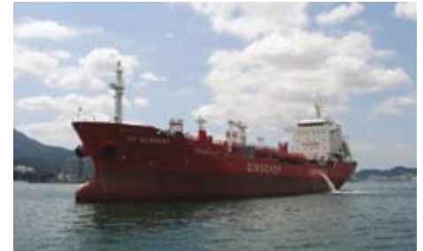
The 13K project has produced forty-five 13,000 ton deadweight chemical tankers with 20 more vessels to be completed
