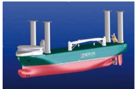
Enercon's E-Ship 1 uses wind energy for propulsion
